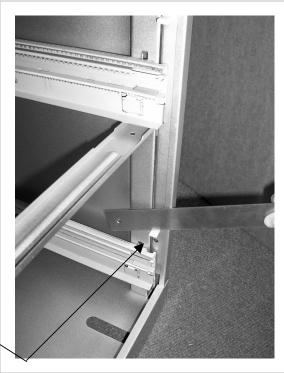
Sometimes the key will turn correctly but all the drawers remain locked. This could be because the locking bar is partially jammed. To open the drawers, a thin metal bar (metal ruler) can be used to push the locking bar down. Insert the metal bar between the drawer front and the side of the carcase, position the metal bar above one of the plastic locking bar tags, and push downwards.
