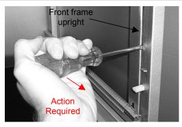
If the locking bar is stiff, try placing a screwdriver between the upright and the locking bar. Working from top to bottom using leverage, ease the screwdriver forwards with reasonable force, this may free the locking bar.
