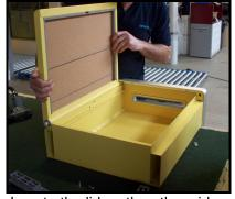
Locate the lid on the other side on the top box and slide the hinge damper into the hole at the front of the unit
