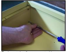
Re-insert the 2 screws at either side of the back of unit to secure the bumpers in place.
