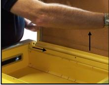
Remove the lid by sliding it towards the back releasing the front hinge and then lift up and away from the unit
