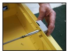
Firstly you would need to remove the lock. If you open the lid you will see this is held in with two screws which if you remove the lock will come away.
