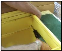
At the back of unit there are 2 screws on either side. Using an appropriate screwdriver remove these. Its best to leave these inside the unit so as not to lose them.
