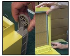
Remove the two top box bumpers at the back of the unit. Take care removing the bumper at the bottom of the lid as the hinge damper locates inside
