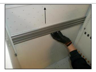
Position the top of the Ladder behind the bottom of the recess and slide upwards until the ladder is at the top of the recess.
