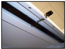
Firstly you will need to remove any drawers or flippers to gain access to the locking mechanism
