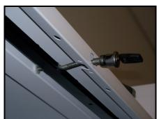
Place the new lock into position with spring clip in place. Ensure the rod is in place in the hole and through the black bar.
