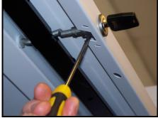
The lock is held in place by a spring clip. To remove place a flat head screwdriver at one end and prise off the lock barrel
