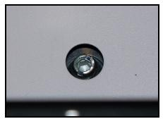
If applicable you will need to remove the bottom one or two drawers to allow access to the bottom of the unit. In each corner there will be access to the feet. They can be adjusted up or down using either an appropriate allen key or flat head screwdriver.
