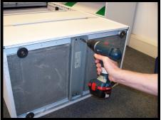
Using an electric or manual screwdriver remove all four screws in each corner of the holding plate and remove the plate. (Please take care as the counterweight may fall out)
