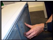
To fit the counterweight insert the edge of the weight underneath the fold on the bottom side of the carcass
