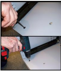
Turn clockwise to raise the foot Turn anti-clockwise to lower
