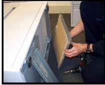
The counterweight can then be removed from the unit.
