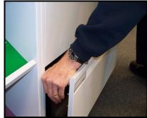
Half close the drawer and push down the front of the drawer on both sides. Again the drawer should click into place on the runners.
