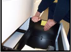
Push down the rear of the drawer on both sides to fully locate the runners tags onto the drawer. You should hear them click into place
