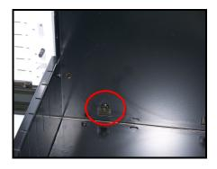
Extend drawer fully, notice that the runners are attached to the side of the drawer by 3 metal lugs
