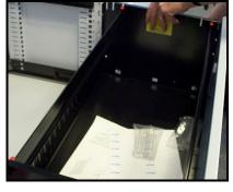
Lift the drawer off the remaining two lugs taking care to support the weight of the drawer.
