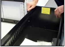
Holding the slide in place lift the back of the drawer upwards and off the rear lug
