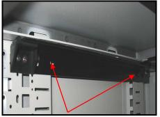
If you wish to remove the flipper mechanism completely, remove the two screws on each flipper rail and remove the rail from unit. Take care to support the rail whilst removing screws.
