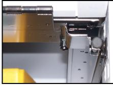
Ensure the slots at the rear of the flipper are correctly located over the rail.
