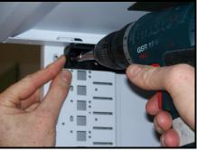
To remove the flipper, remove the two screws holding in the stopper on both sides.
