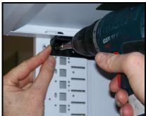
Fix the stopper into place by inserting the two screws.
