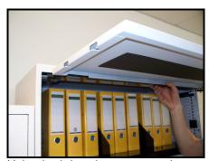
Using both hands to support the front and back, slide the flipper out and away from the unit.
