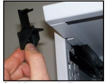
Carefully remove the flipper stops by sliding out over the flipper. Take note of the way in which they fit for ease of refitting.
