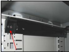
Open the flipper fully. You will see the flipper rail on either side of the unit. There is a black plastic stopper on the front end held in by two screws.
