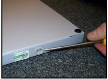
If the locking bar has fallen inside the door you will need to retrieve it. Remove the plastic locking bar guide from either end of the cupboard door using a flat head screwdriver.
