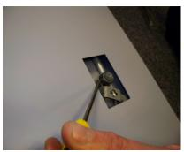
Using a flat head screwdriver unclip the spring clip which holds the lock in place. The lock can then be removed from the door completely.
