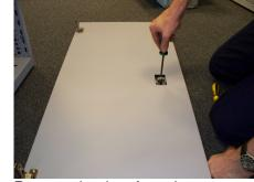
Remove the door from the cupboard and lay down on its front. Using an appropriate screwdriver remove the screw in the back of the lock and move the locking bar away from the lock
