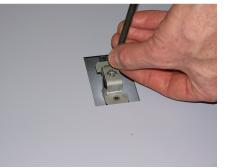
Replace the washer and screw into the back of the lock
