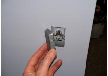
If the locking bar has fallen inside the cupboard, to retrieve it firstly you would need to remove the lock from the door. Remove the protective cover to reveal the lock mechanism
