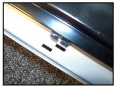
Reattach the runners by inserting the lugs into the corresponding holes and sliding towards the side
