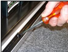
Ensure the tambour doors are in the fully open position. You will see black plastic runners top and bottom. Using a flat head screwdriver release the end clip in the centre of the cupboard
