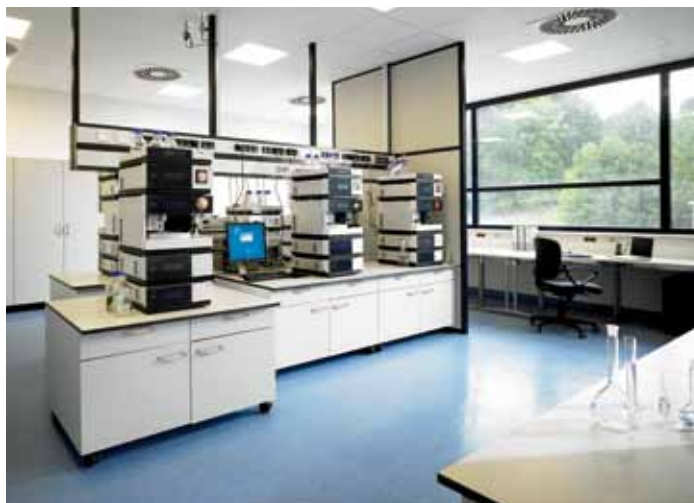
Mobile cabinets for HPLC installations. Soundproofed walls shield the area for carrying out desk work
